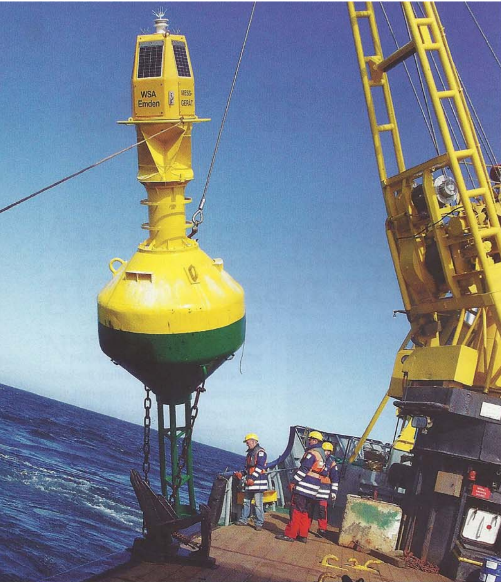
Above: Three-tonne buoy used to moor T-PODs, C-PODs and other oceanographic equipment at a control location.
